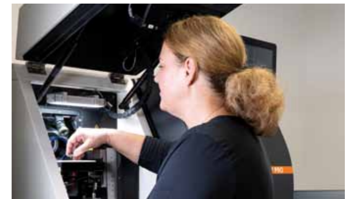
Ultra-thin samples for nanoanalytics can be produced faster and more reliably using the microPREP™ device developed by Fraunhofer IMWS.
